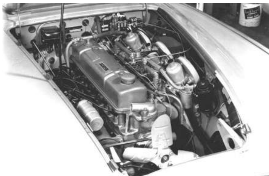
Rare factory publicity photo of tri-carb installation, marked "Confidential until Sept.20." (1960?)
